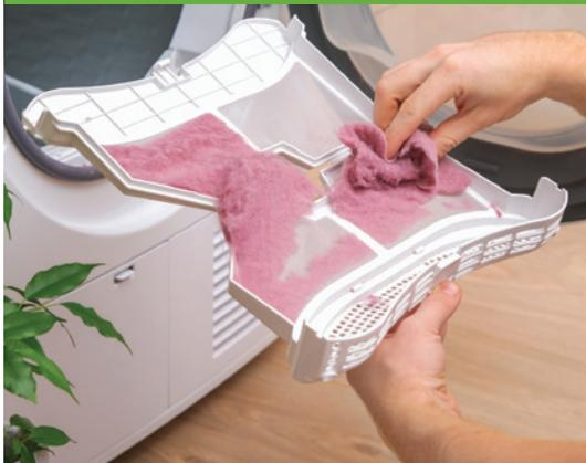
Lengthen the life of your clothes dryer with regular cleanings. Clean the lint filter after every load, which improves air circulation and safety. Check the lint trap opening to ensure it's clean. Use a vacuum to remove any lint that's fallen inside the opening.
